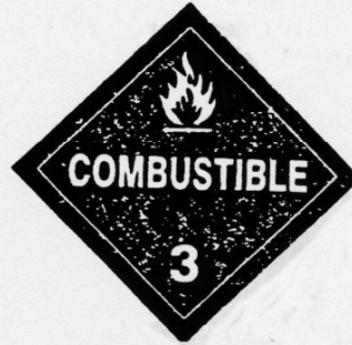
COMBUSTIBLE Background color: red Symbol, text, numerals and border: white On a COMBUSTIBLE placard with a white bottom the numerals must be in red or black. The words "FUEL OIL" may be used in place of the word "COMBUSTIBLE"
