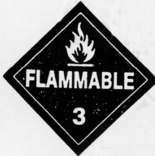
FLAMMABLE Background color: red Symbol, text, numerals and border: white The word "GASOLINE" may be used in the place of "FLAMMABLE"
