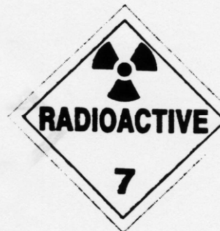
RADIOACTIVE Background color: white in the lower portion with a yellow triangle in the upper portion Symbol, text, numerals and border: black
